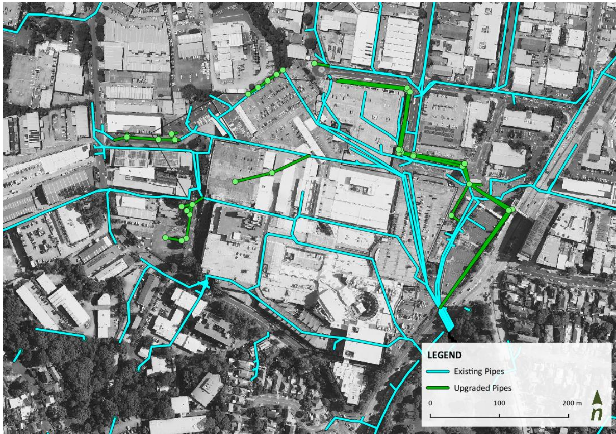
Figure 25. Additional stormwater infrastructure modelled
